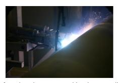
The Metallisation ARC528E system consists of an ARC528E servo driven pistol, 5m supply package and a 450 amp switched voltage energizer with inbuilt closed loop wire speed control unit. The aluminium wire is dispensed from production packs, which reduces downtime
