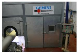
Gemini has a purpose built, fully automated, computerised metal spray facility at its Montrose base, which was designed and installed by Metallisation. The pipe manipulation system is flexible and can cater for different pipe sizes, enabling a full range of pipes to be sprayed using just one machine.
