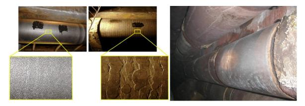
The image on the left, shows a laser clad surface after 118 ktonnes. The image in the middle, shows a sub arc welded surface after 63 ktonnes.
