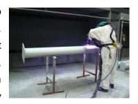
different shaped structures. It can be a little messy with the dust produced but this has been easily overcome with some minor planning changes. The dust is also easy to clean up as over spray does not stick to the surrounding area. The operators have been surprised by the amount of work achievable and have found that it's not as wasteful of coating material as they previously thought it would be.
