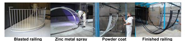
The finished thickness of coating is in the region of 250-300 microns. As per the European standard EN ISO 14713, this coating system has an expected life to first maintenance of 20 years plus in many environments. Professional Coatings guarantees that the powder coating will not flake off. Its confidence in this guarantee has been increased by the higher quality of bond achieved with powder coating over metal spray as opposed to conventional hot dip galvanising.
