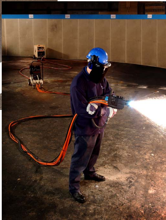
170 system spraying from MIG reels with 10m from energiser to site trolley and 10m from site trolley to pistol
